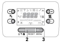
■ The display will show CO and the ▲, ▼, ▶ and ✓ icons will light up. The boiler operates at the maximum heating output.
