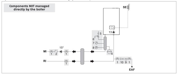
Layout 4: circuit with boiler connected to DHW tank and heating system via separator
