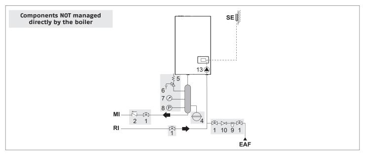
Layout 2: circuit with boiler directly connected to heating system and DHW tank (check that the pump discharge head is sufficient to ensure adequate circulation)
