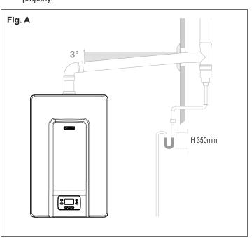
For changes of direction, use a T-fitting with inspection plug which allows easy periodic cleaning of the pipes.
