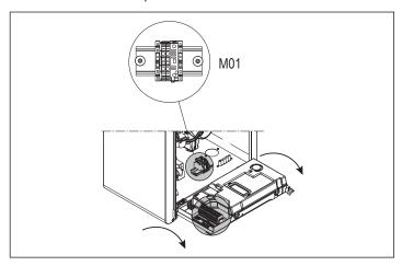
• insert the supply cable (not supplied) in the cable grommet underneath the bracket, then connect it as shown in the figure and fix it in place using the tear-off tie, tightening it firmly.
