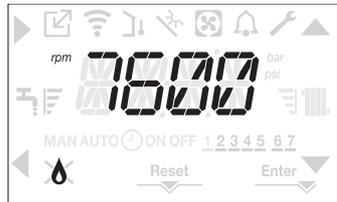
The boiler will work at the maximum output.
