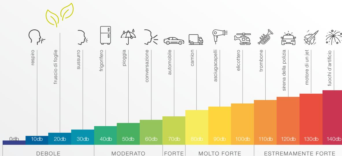
SCALA DELLE EMISSIONI SONORE PERCEPITE IN DB CON ESEMPI DI LIVELLI COMPRESI TRA 0 E 140 DB
