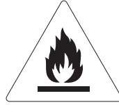
Caution: Risk of fire/ flammable materials
